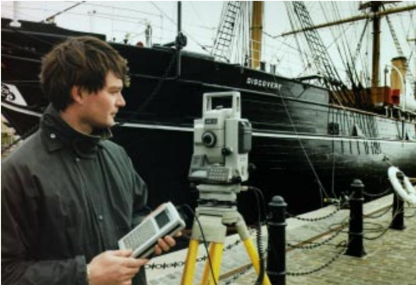
*Built in 1898 in Scotland, the Discovery was used by Captain R. Scott to explore Antarctica. When launched, it was the strongest ship ever built; still, it was trapped in ice for more than two years during its exploration. Finally brought back to Scotland in 1986, Discovery was the subject of a distortion survey carried out by Warner Land Surveys of Oxford, England, using the NET2 3-D Electronic Total Station.*
